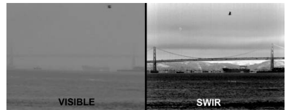
The visible light image (left) shows mostly fog; the SWIR image (right) reveals detail through the fog. SWIR technology detects reflected light at wavelengths that the human eye cannot see, in bands on the electromagnetic spectrum between the visible and thermal. ( https://spinoff.nasa.gov/Spinoff2010/ip_2.html )
